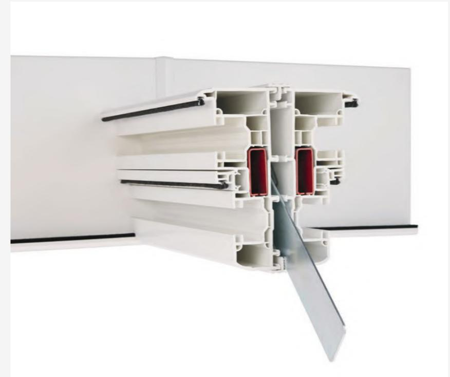
A coupling nut can be used as an alternative and simpler way to connect profiles. This 'invisible' fixing sits between the outerframe of each window so there's no need to drill through the visible frame. A concealed coupling cover finishes the job off nicely, both inside and out.
