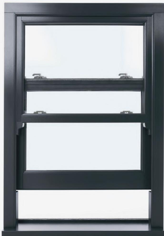
A sculptured 146mm outerframe and sculptured sash frame provide the look of timber, with all the benefits of PVCu. Balanced, slim sightlines and a square travel stop cover, maximise light and provide an elegant timber-like aesthetic. Whilst the interlock between the top and bottom sash increases weather performance and security, providing customers with peace of mind.
